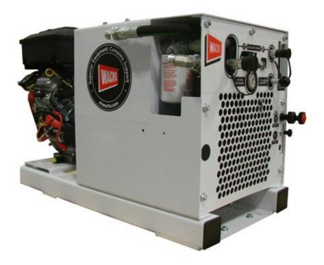
The Wachs HPU-750 is designed to supply hydraulic power to the ERV-750, and TM-7 valve operators, or any HTMA Class II hydraulic tool. Equipped with a Briggs & Stratton 16 HP Vanguard V-Twin OHV gasoline engine driven hydraulic power supply with dual auxiliary circuits, electric start and electric fan driven oil cooler.
